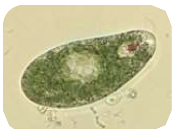
MLSS sample- Some Nocardia present but not the high levels shown in the foam.
