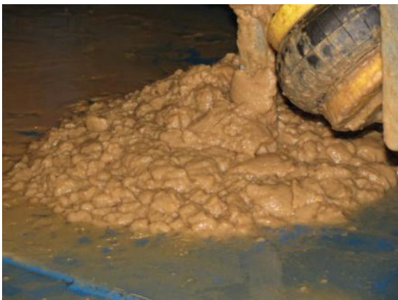
Zooglea is also very hard to dewater, and adds significant weight to your solids. Polymers cannot help Zooglea, and adding chlorine to your aeration basins with Zooglea will only make it worse.
